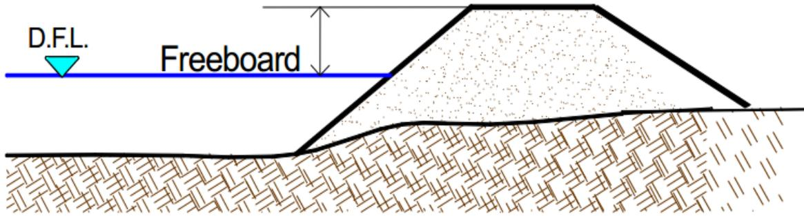
$$\text{Dike height} = \text{Design flood level} + \text{Freeboard}$$
