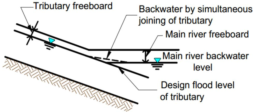
**Figure 7.** Free board due to backwater effect
