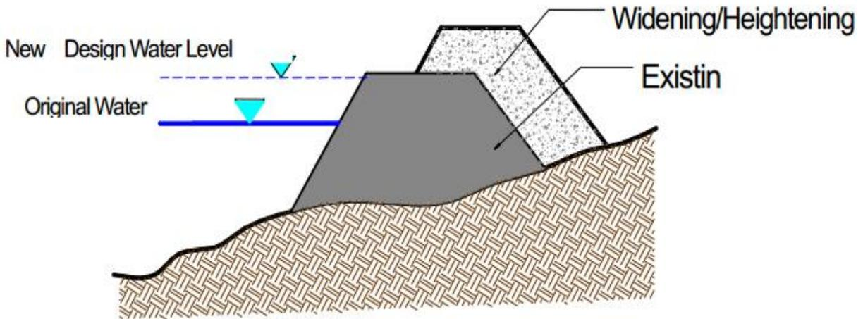
**Figure 4.** Widening and heightening of existing dike
