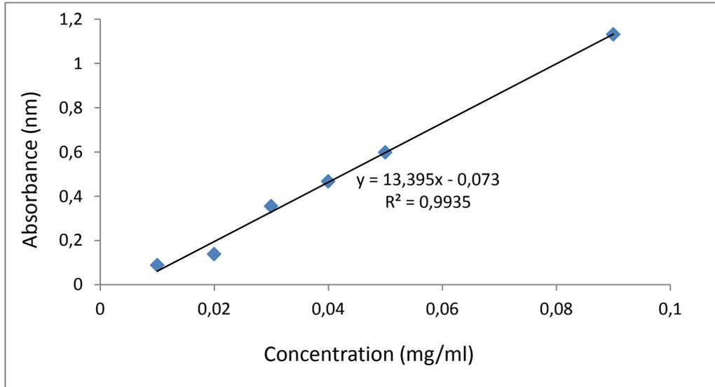
**Figure 1.** Calibration curve of glucose standard for determination of total reducing sugar content
