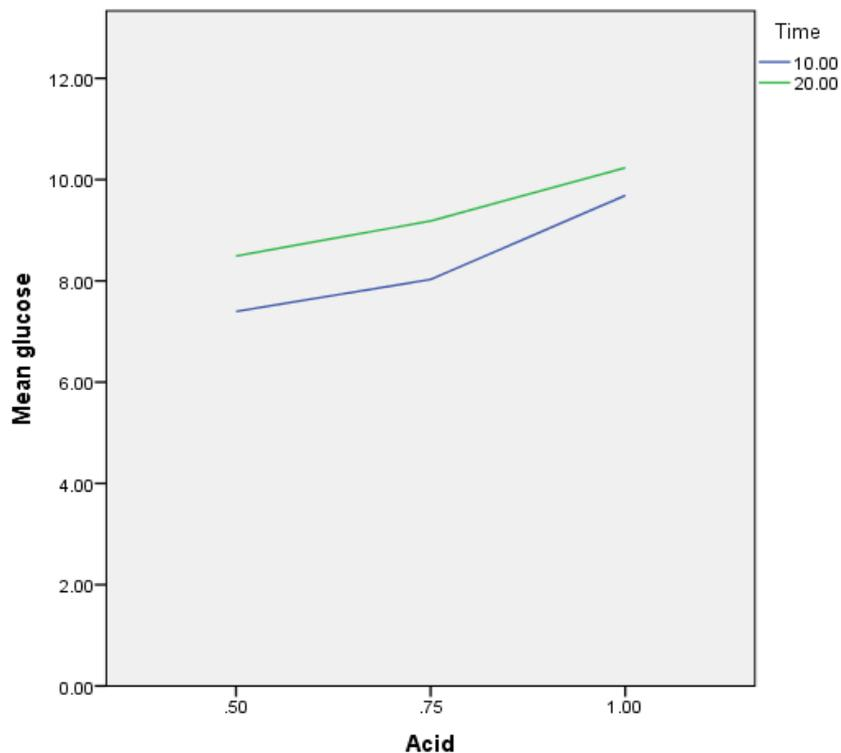
**Figure 2.** Analysis of effect of different concentration of sulphuric acid and treatment time on release of glucose during hydrolysis.
