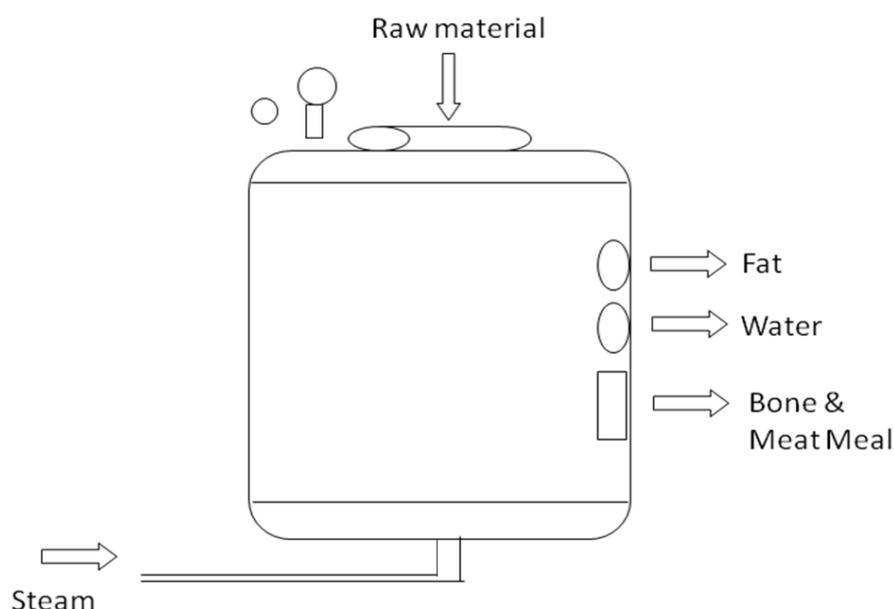
**Figure 2.** The Sketch of the wet rendering process
