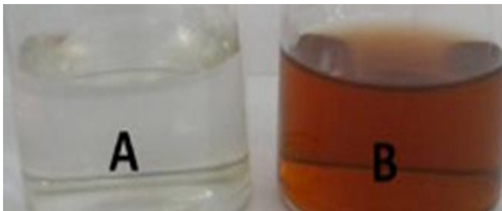
Figure 2. Mycosynthesis of silver nanoparticles using Aspergillus terreus aqueous extract treated with \text{AgNO}_3 solution at room temperature: (A) Silver nitrate ( \text{AgNO}_3 ) solution, (B) formation of silver nanoparticles using Aspergillus terreus aqueous extract.
