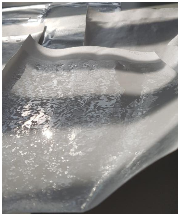
Figure 2. Paper coated with Methocel™ containing polylysine (on the surface of Topscreen layer)
