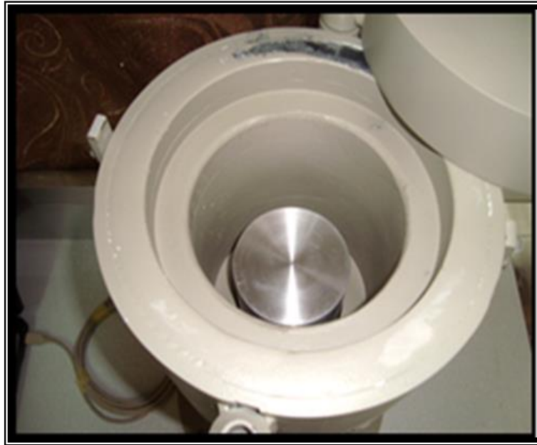
Figure 2. Detector position in the shielding.
