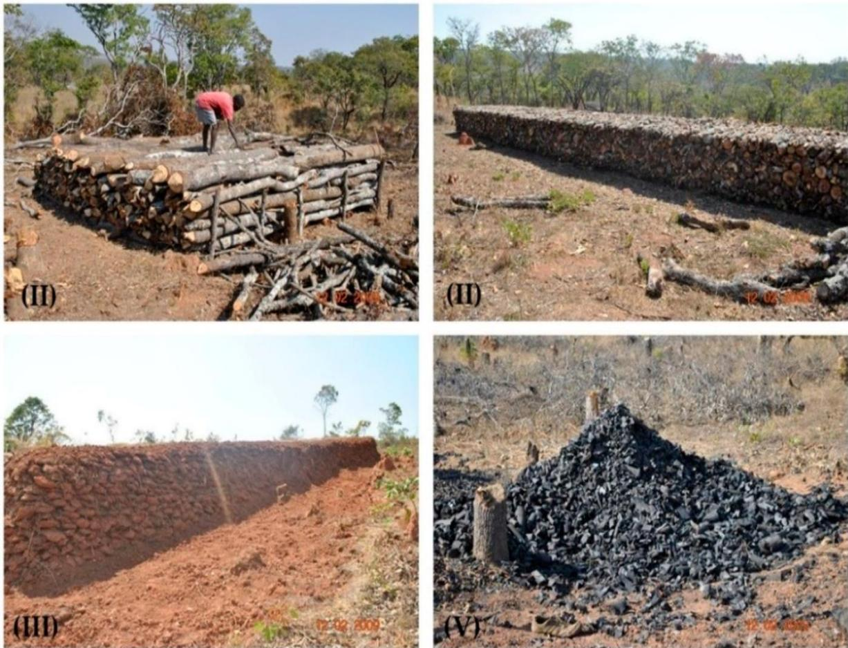
**Fig. 1.** Processes of charcoal production by traditional earth kiln. Upper images (II) show the process of log piling into clamp, and the lower left image (III) shows covering of the clamp with dung and soil lumps, while the lower right image (V) shows the harvesting of charcoal and packaging it into bags. The steps number (I, IV) is not represented in this figure.
