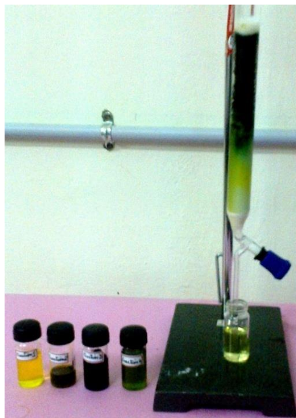
Figure 2. Column chromatography: separation of fraction from Pn -MLEFr
