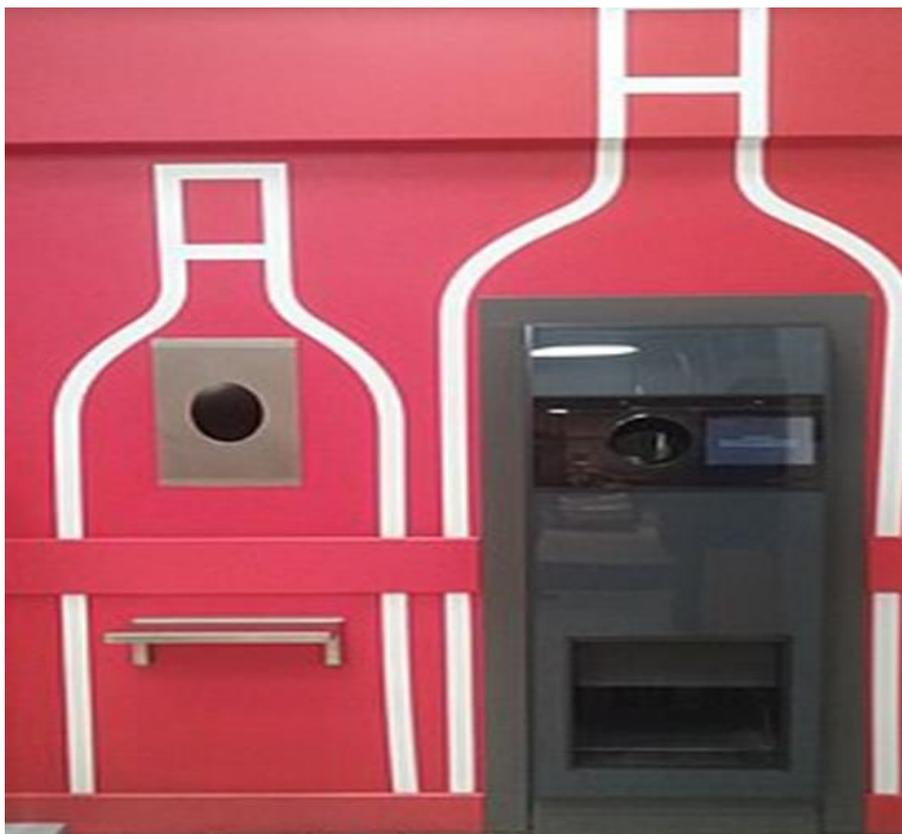
**Figure 5.** Reverse vending waste machine (Layton, 2009)
