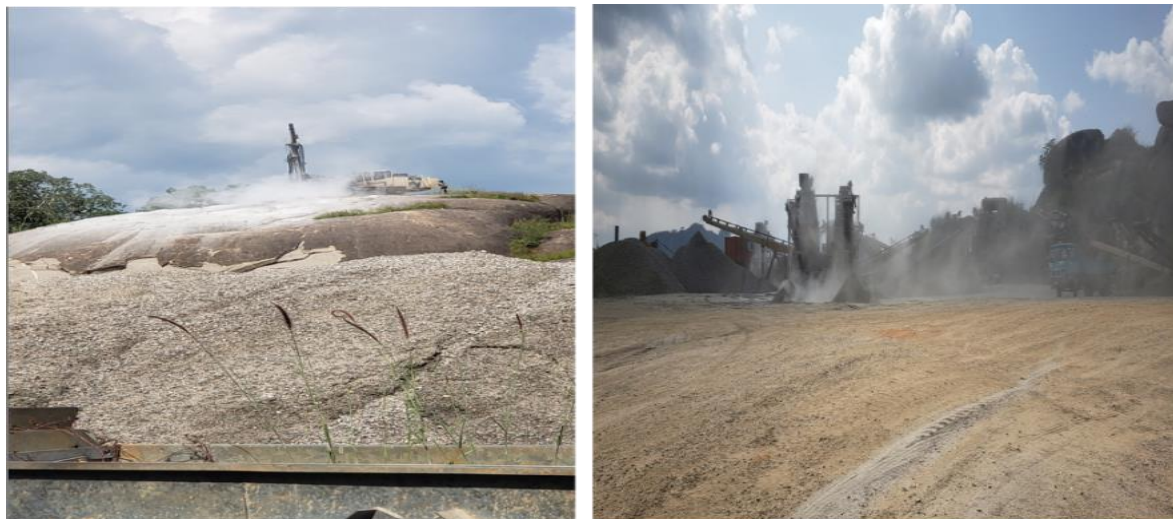
Figure 6. Dust Produced during Crushing and Drilling at Quarry Sites
