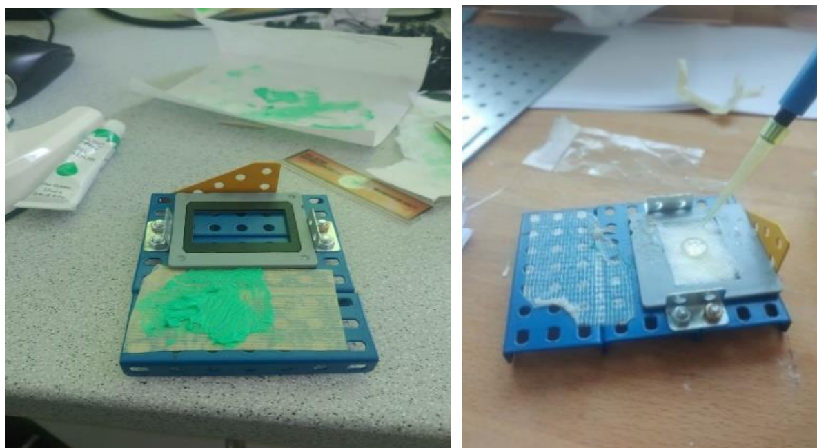
Figure 1. (a) Self-made manual multilayer material fabrication kit (MMF), and (b) PP layer covered with gelatin binder.
