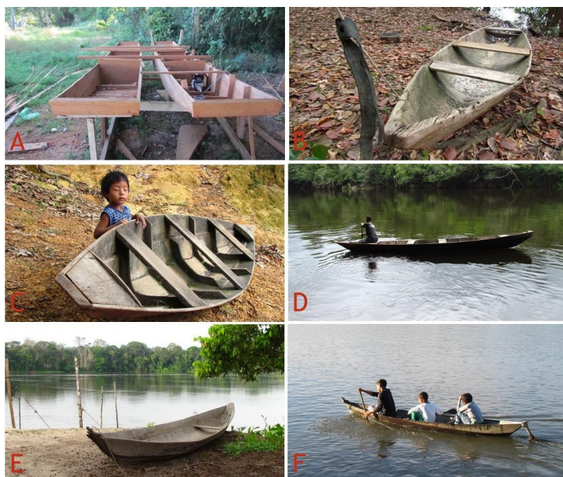
Figure 6. (A) Detail of a boat being built by an Arara Indigenous person using itaúba planks ( Mezilaurus itauba ); (B) (C) (D) Tenharim paddle canoes; (E) Kayabi paddle canoe (Photos by Fabio Rossano Dario).
