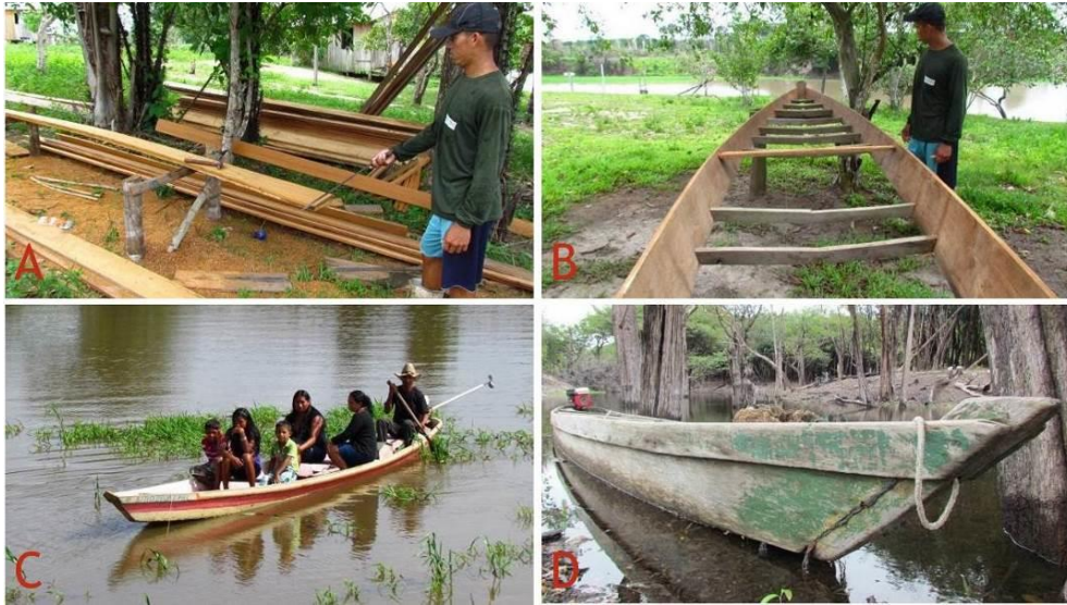
Figure 3. (A) and (B) Detail of a canoe being built by a Mura indigenous person in the Aparecida do Correnteza village, in the Rio Urubu Indigenous Land; (C) and (D) Canoes built by the Mura indigenous people, with plank structures and equipped with a 6.5 Hp motor known as a "rabeta." (Photos by Fabio Rossano Dario).
