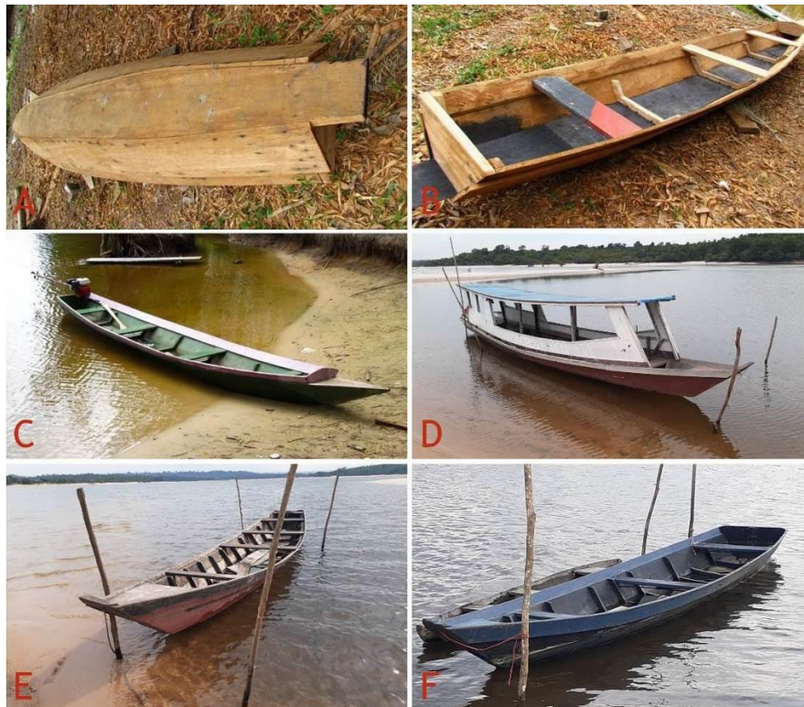
Figure 4. (A) Hull construction of a canoe made with wooden planks; (B) The canoe is nearly finished, with the side braces to hold the planks already in place, as well as the seating benches; (C) Detail of a canoe equipped with a 6.5 HP rabeta (long-tail) motor; (D) (E) (F) Detail of canoes used by riverside dwellers in the Amazon (Photos by Fabio Rossano Dario).
