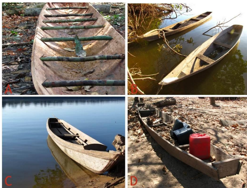
Figure 5. (A) Canoe documented in the Apiaká Indigenous Land, carved from a single trunk of jacareúba wood ( Calophyllum brasiliense ); (B) Apiaká paddle canoe docked on the banks of the Teles Pires River; (C) Kayabi paddle canoe docked on the banks of the Teles Pires River; (D) Bororo paddle canoe, documented in the Aijeako village, in the Meruri Indigenous Land, built with jequitibá wood ( Cariniana legalis ) (Photos by Fabio Rossano Dario).
